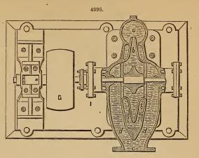
air from getting through the stuffing box, the latter is put in communication with the delivery column by means of a pipe constantly filled with water; and, in case the air should get into the centre through the suction-pipe, in order to fetch the pump again without stopping it, two holes are provided which put the centre of the wheel in communication with the interior of the chamber into which the water is forced; this forces the air to escape.
